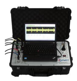
The PDiagnostic is a portable system that utilizes Ultra-High Frequency (UHF), Acoustic Emissions (AE), High-Frequency Current Transformer (HFCT), and Transient Earth Voltage (TEV) sensors to detect, analyze, and locate the PD signals in real time for a multitude of medium and high voltage electric power equipment.
